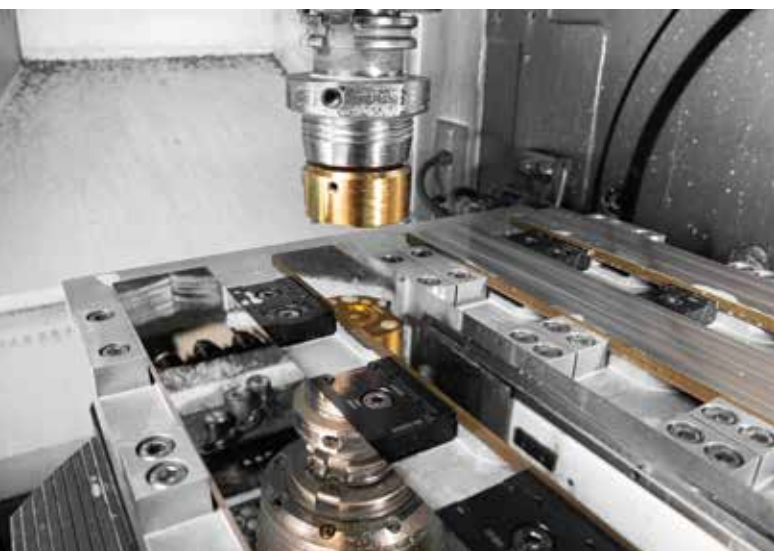
High-polish milling produces perfect flatness and mirror-like surface finishes measured in nanometres.
