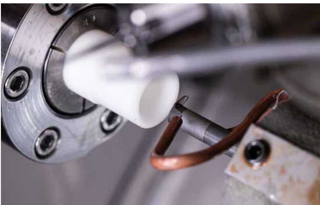
When machining the ring from an abrasive plastic, a PCD grade is essential.
