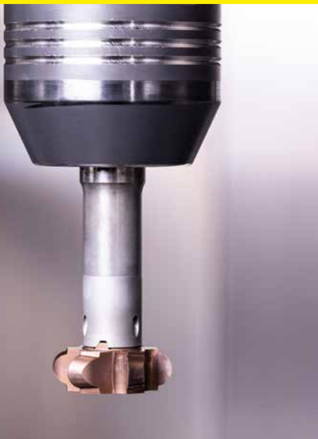
Götz machines fillets using an end mill with a solid carbide insert.
