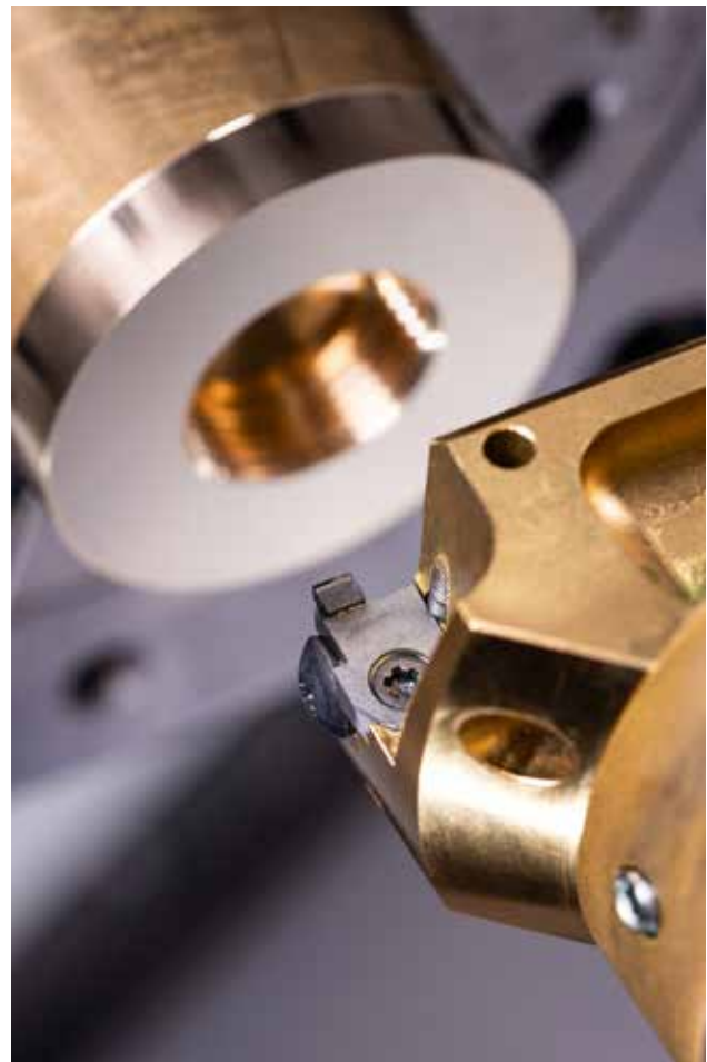
An MCD-equipped S117 system is used to machine the end faces.
