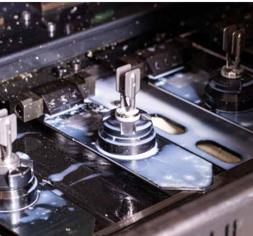
The M fork is used in level indicators.
