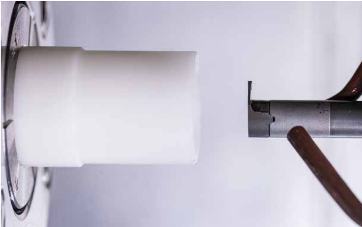
The Mini type HORN system is used for boring.
