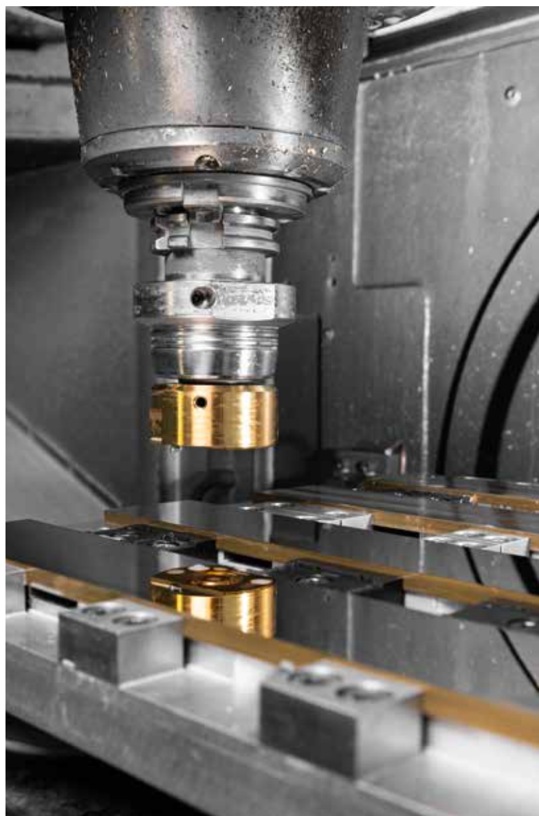
High-polish milling produces perfect flatness and mirror-like surface finishes measured in nanometres.
