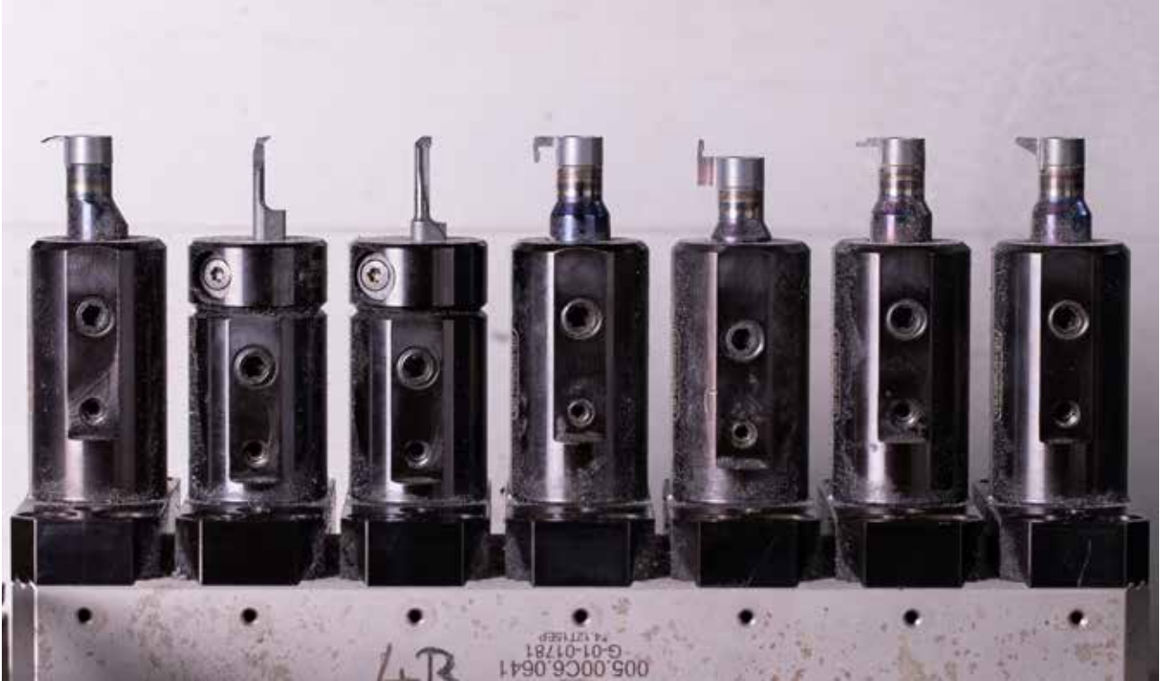
Tools are mounted in line on a platen for each machining operation.
