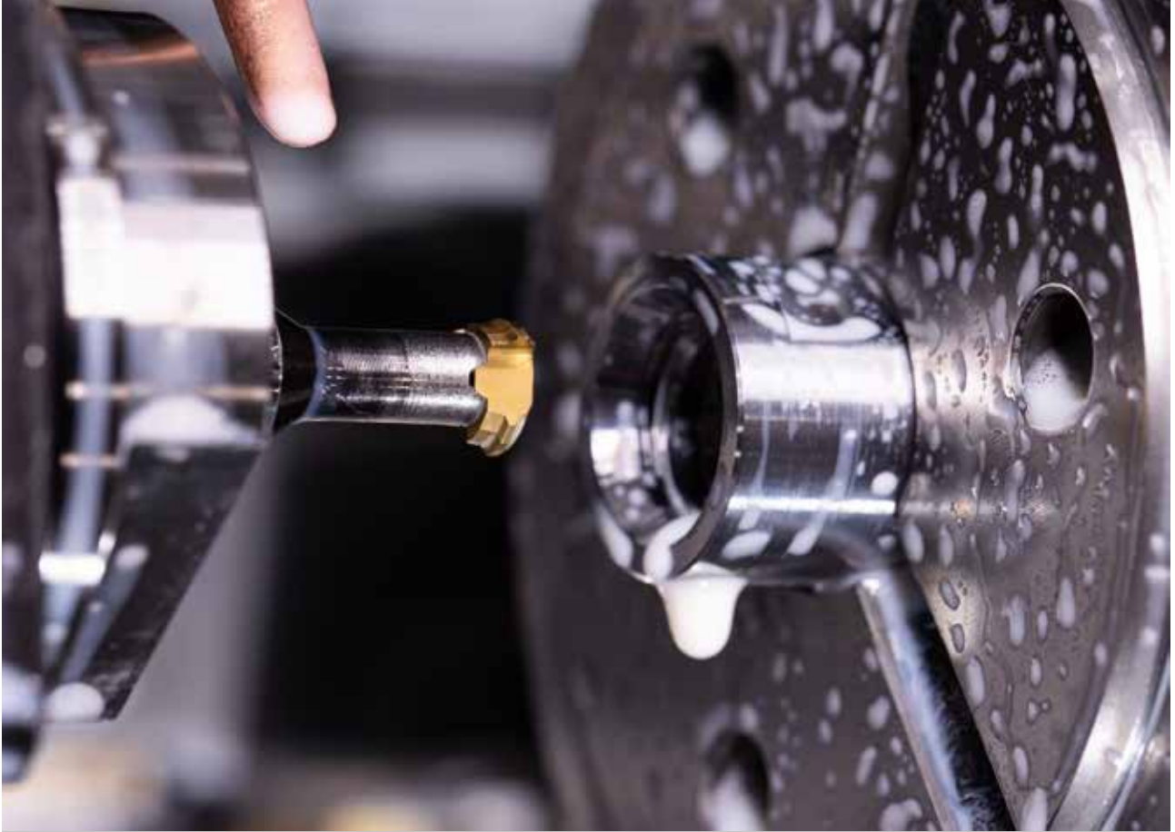
A type 306 insert is used for milling the precision thread.
