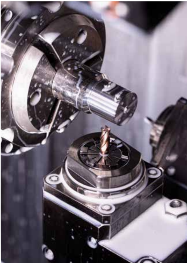
Milling of spanner flats with the HORN DS system.
