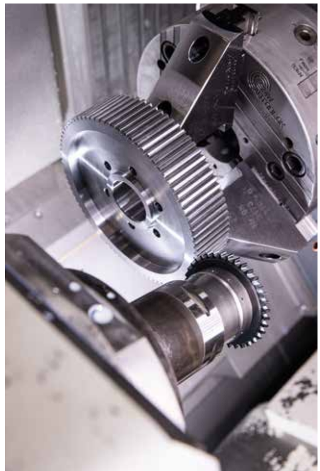
The disc carrier is used in a clutch/brake combination.
